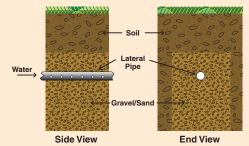
Water flows out of the laterals into a bed of gravel or sand which acts as a final filter before the water enters the ground.
